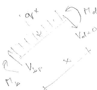
$$M_a = M_b + V_{bp} X - Q X$$
