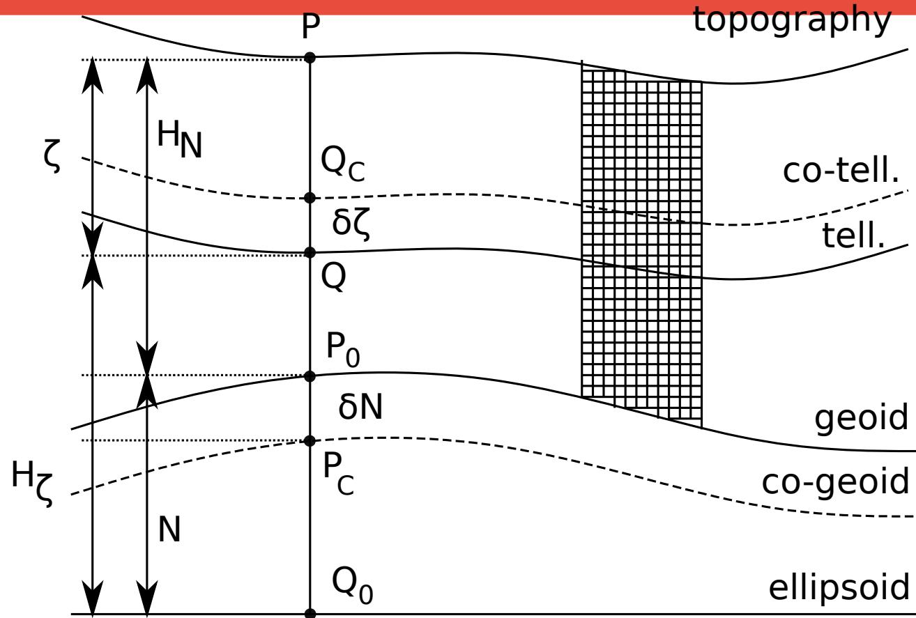
$$N - \zeta = \frac{\bar{y} - \bar{g}}{\bar{y}} \cdot H \approx \frac{\Delta g_P^{BO}}{\bar{y}} \cdot H + \frac{V^T(P_0) - V^T(P)}{\bar{y}}$$
