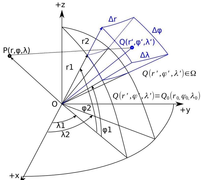
$$V^*(P(r, \varphi, \lambda)) = G\rho \int_{r_1}^{r_2} \int_{\varphi_1}^{\varphi_2} \int_{\lambda_1}^{\lambda_2} \frac{r'^2 \cos \varphi' dr' d\varphi' d\lambda'}{\sqrt{r'^2 + r^2 - 2rr'(\sin \varphi \sin \varphi' + \cos \varphi \cos \varphi' \cos(\lambda' - \lambda))}}$$
