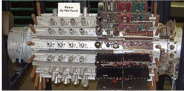
Figure1: Mercury delay line memory of UNIVAC I ( https://en.wikipedia.org/wiki/UNIVAC_I )
