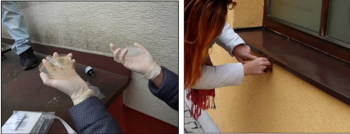
Fig. 7: Sampling by tape from the strata under the plaster. Fig. 8: Sampling of surrounding façades- without insulation- for comparison.
