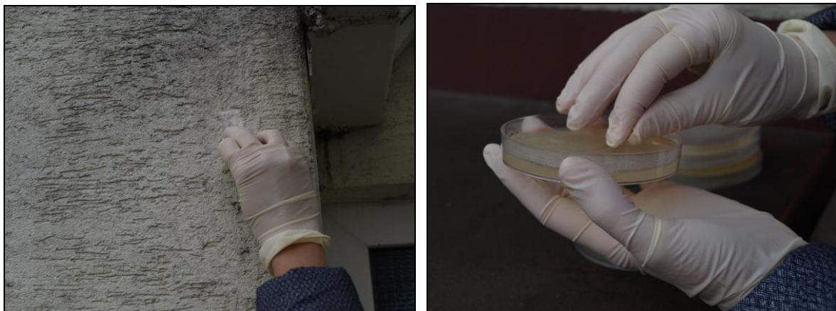
Fig.3, 4: Taking of samples with sampling tape (Fungitape) from the surface of contaminated plaster. (Antošová, Piecková)
