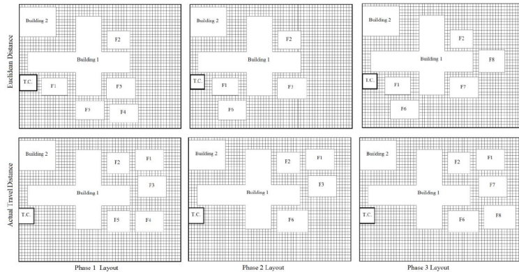
Figure 5. Comparison of layouts from linear distance and actual travel distance driven optimization
