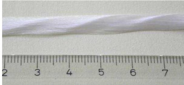
Figure 5.15: Waves in the tested yarn
