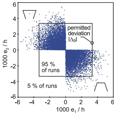
Fig. 5. MC runs, Case 2, Class 2,  $\sigma_{e1} = \sigma_{e2} = h/670$ .
