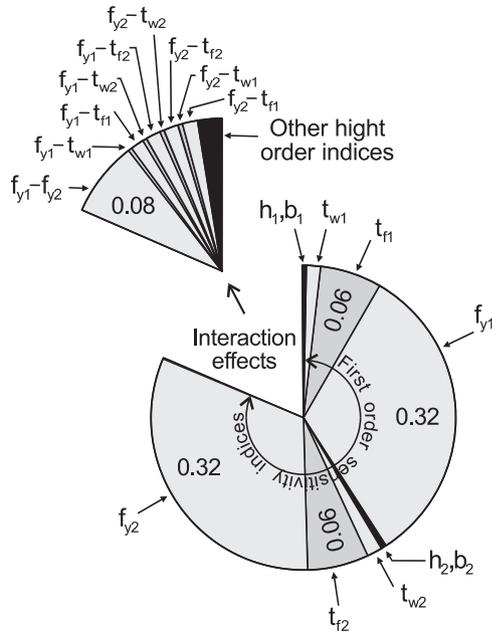
Fig. 8. Sensitivity analysis for  $\bar{\lambda}=0$ .
