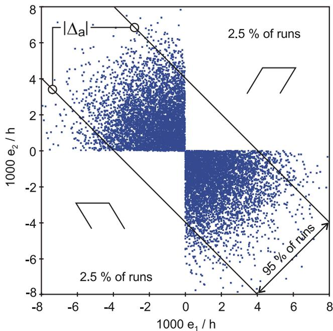
Fig. 6. MC runs, Case 2, Class 1,  $\sigma_{e1} = \sigma_{e2} = h/430$ .
