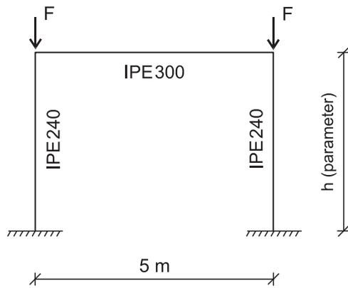
Fig. 1. IPE-section symmetric portal frame.
