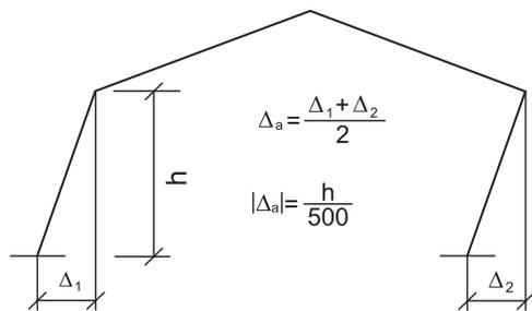
Fig. 2. Inclination of a single storey portal frame building.
