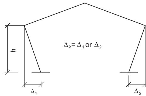
Fig. 3. Inclination of each column.
