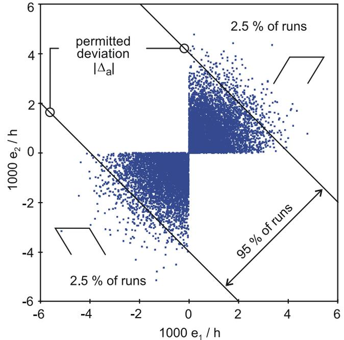
Fig. 4. MC runs, Case 1,  $\sigma_{e1} = \sigma_{e2} = h/790$ .
