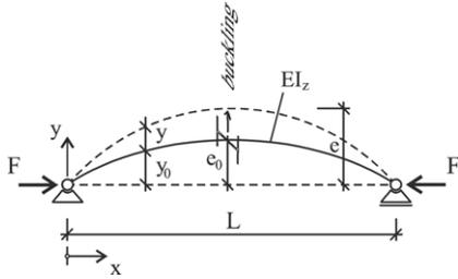
Fig. 1. Buckling of the member with IPE cross-section.
