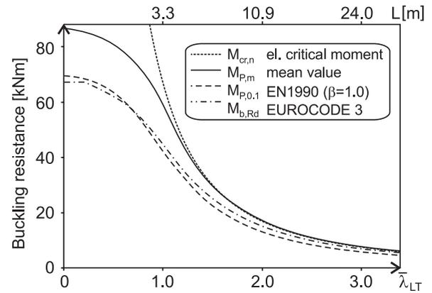
Fig. 13 – Statistical analysis of inelastic buckling resistance  $M_P$ .
