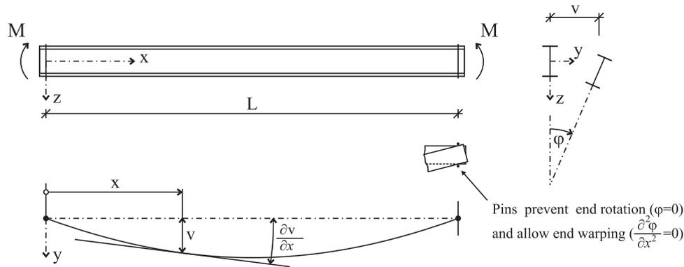
Fig. 2 – Buckling of simply supported IPE-beam.
