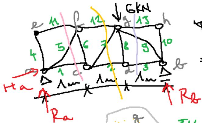
$$\begin{aligned} \sum M_a = 0 & \quad H_a \cdot 0 + R_a \cdot 0 - 6 \cdot 2 + R_b \cdot 3 = 0 \Rightarrow R_b = 4 \text{ kN} \\ \sum M_b = 0 & \quad H_a \cdot 0 + R_a \cdot 3 + 6 \cdot 1 + R_b \cdot 0 = 0 \Rightarrow R_a = 2 \text{ kN} \\ \sum F_x = 0 & \quad H_a = 0 \\ \sum F_y = 0 & \quad 4 - 6 + 2 = 0 \quad \checkmark \end{aligned}$$
