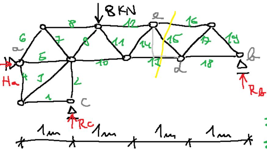
$$\begin{aligned} \sum M_a = 0 & \quad H_a \cdot 0 + R_c \cdot 1 - 8 \cdot 1,5 + R_b \cdot 4 = 0 \Rightarrow R_b = +1,335 \text{ kN} \\ 1 \text{ m} \quad \sum M_b = 0 & \quad -R_c \cdot 3 + 8 \cdot 2,5 + H_a \cdot 0 = 0 \Rightarrow R_c = 6,6 \text{ kN} \\ \sum M_c = 0 & \quad -H_a \cdot 1 + R_c \cdot 0 - 8 \cdot 0,5 + 1,335 \cdot 1 = 0 \Rightarrow H_a = 0 \\ 1 \text{ m} \quad \sum F_x = 0 & \quad H_a = 0 \quad \checkmark \end{aligned}$$
