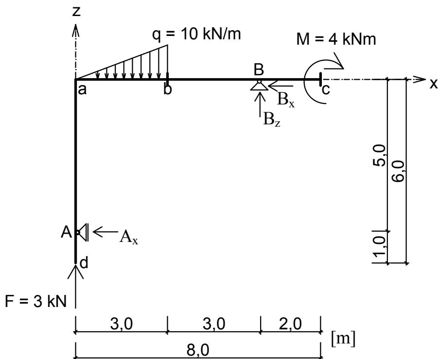
$$A_x = 7,6 \text{ kN} \quad B_x = -7,6 \text{ kN} \quad B_z = 12,0 \text{ kN}$$
