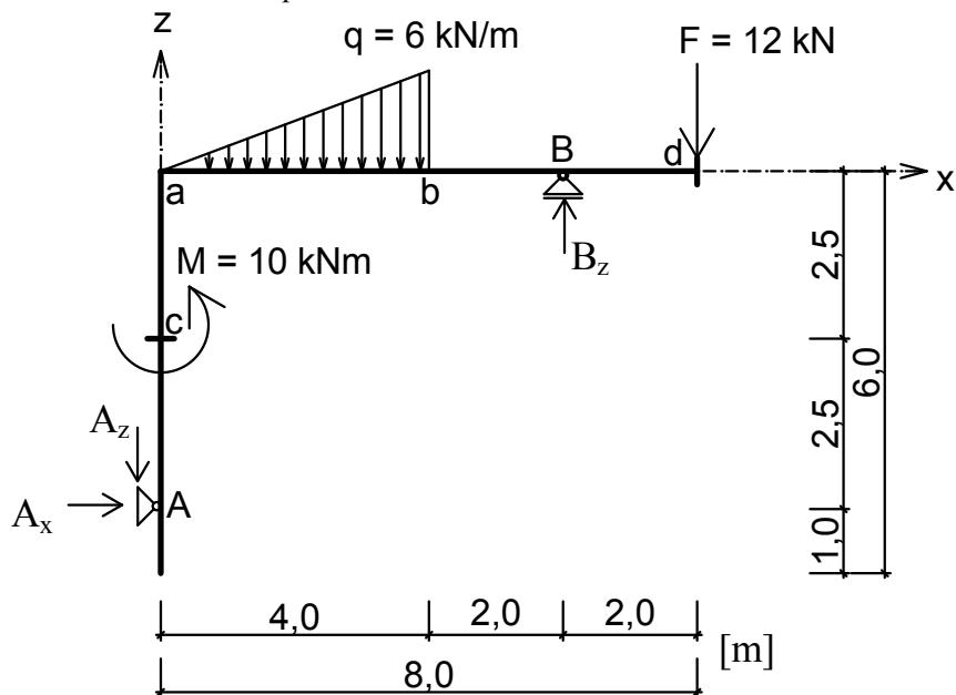
$$A_x = 0,0 \text{ kN} \quad A_z = -4,333 \text{ kN} \quad B_z = 19,667 \text{ kN}$$
