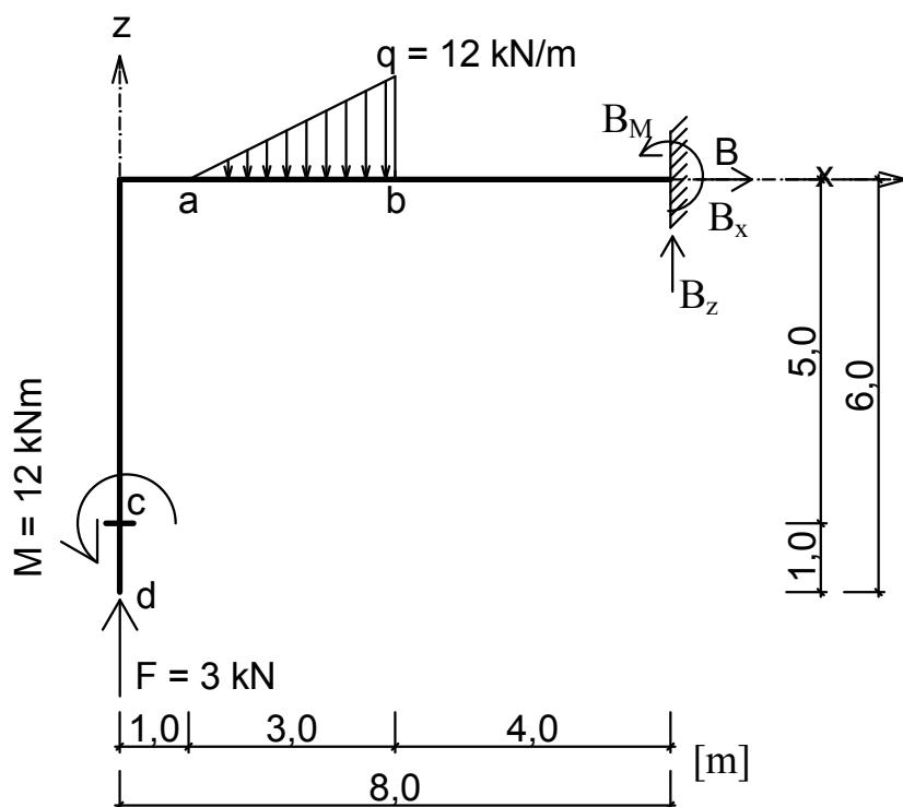
$$B_x = 0,0 \text{ kN} \quad B_z = 15,0 \text{ kN} \quad B_M = -78,0 \text{ kNm}$$
