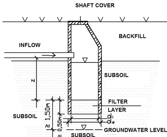
*Fig. 1: Infiltration shaft*
