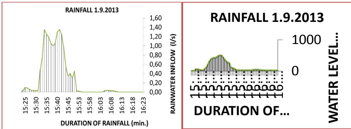
Fig. 7: Example of rainwater infiltration process (water level changes at the bottom of the shaft A) depending on rainwater inflow – rainfall 1.9.2013
