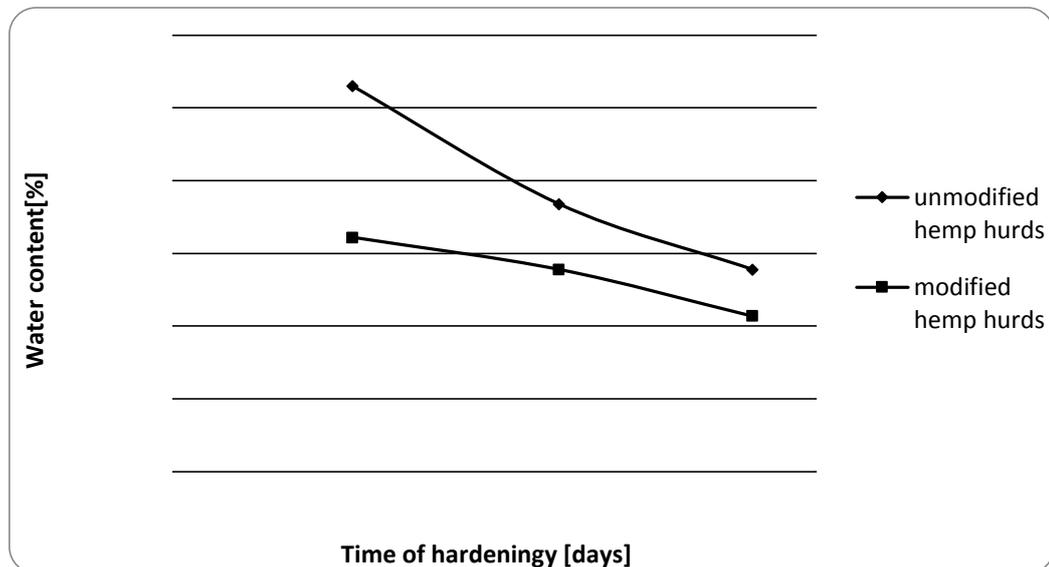
Fig. 4: Dependence of water content in biocomposites on time of hardening
