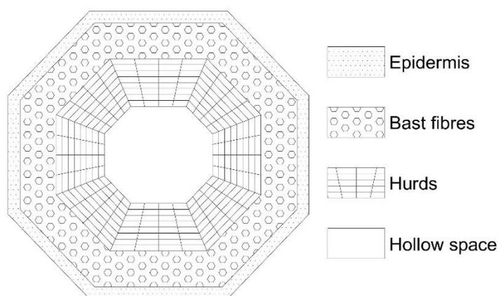
*Fig. 1: Hemp stem – cross section*
