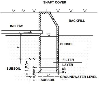
Fig. 1: Infiltration shaft
