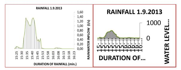
*Fig. 7: Example of rainwater infiltration process (water level changes at the bottom of the shaft A) depending on rainwater inflow – rainfall 1.9.2013*
