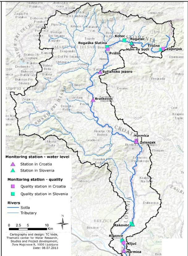
Figure 3: Monitoring stations of water level and monitoring station of water quality
