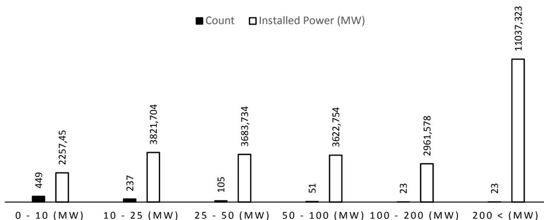
Fig. 3. Distribution of number of HPPs and total installed power by different classifications (EMRA).
