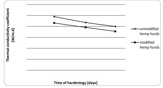
Fig. 3: Values of biocomposites thermal conductivity coefficient in dependence on time of hardening
