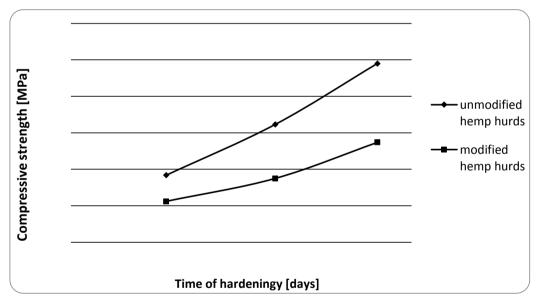
Fig. 2: Dependence of biocomposites compressive strength on time of hardening
