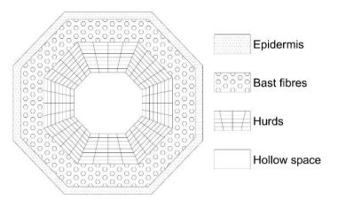
Fig. 1: Hemp stem – cross section
