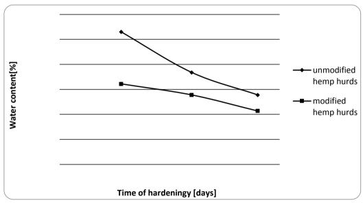
Fig. 4: Dependence of water content in biocomposites on time of hardening
