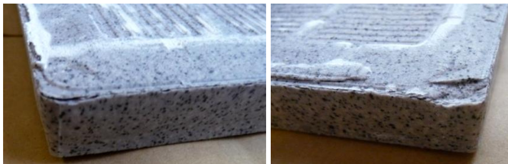
Fig. 6 Examples of new pressed ‘gres’ tiles with damages on side edges.
