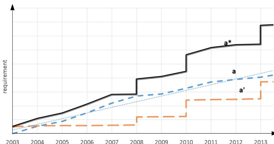
Fig. 2: Reference functions for buildings  $a$  – reference function for social aspects with linear trend function  $y = 4,2064x - 8423,1$   $R^2 = 0,9747$ ;  $a'$  – reference function for technical/legal aspects;  $a^*$  – added together reference functions (social aspects and technical/legal aspects) (according to [9]).
