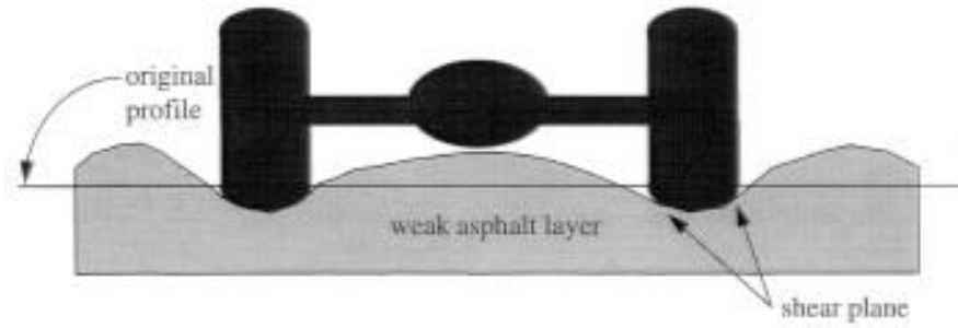
Fig. 3: Rutting in asphalt layers
