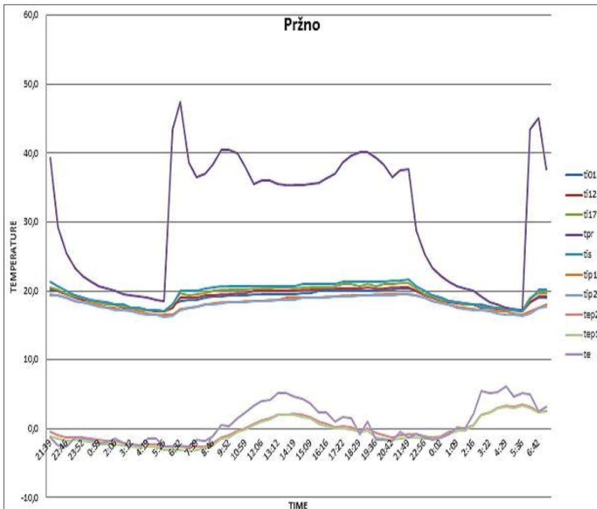
Fig. 5: Temperature curves in the interior of the critical room
