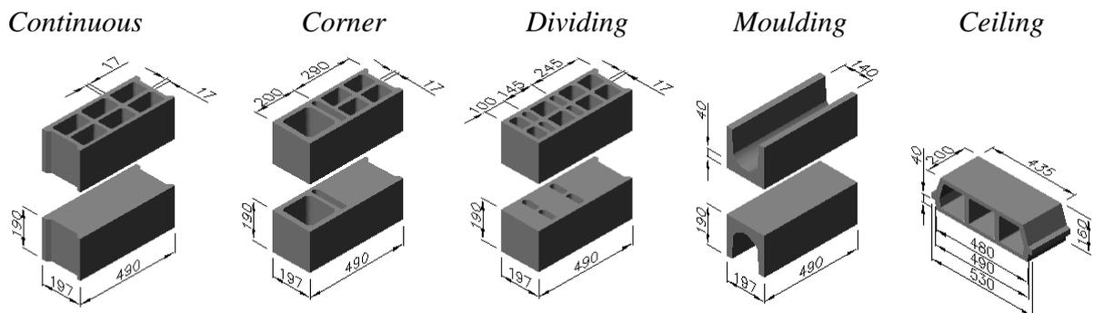
*Fig. 2: Main production range of concrete blocks*
