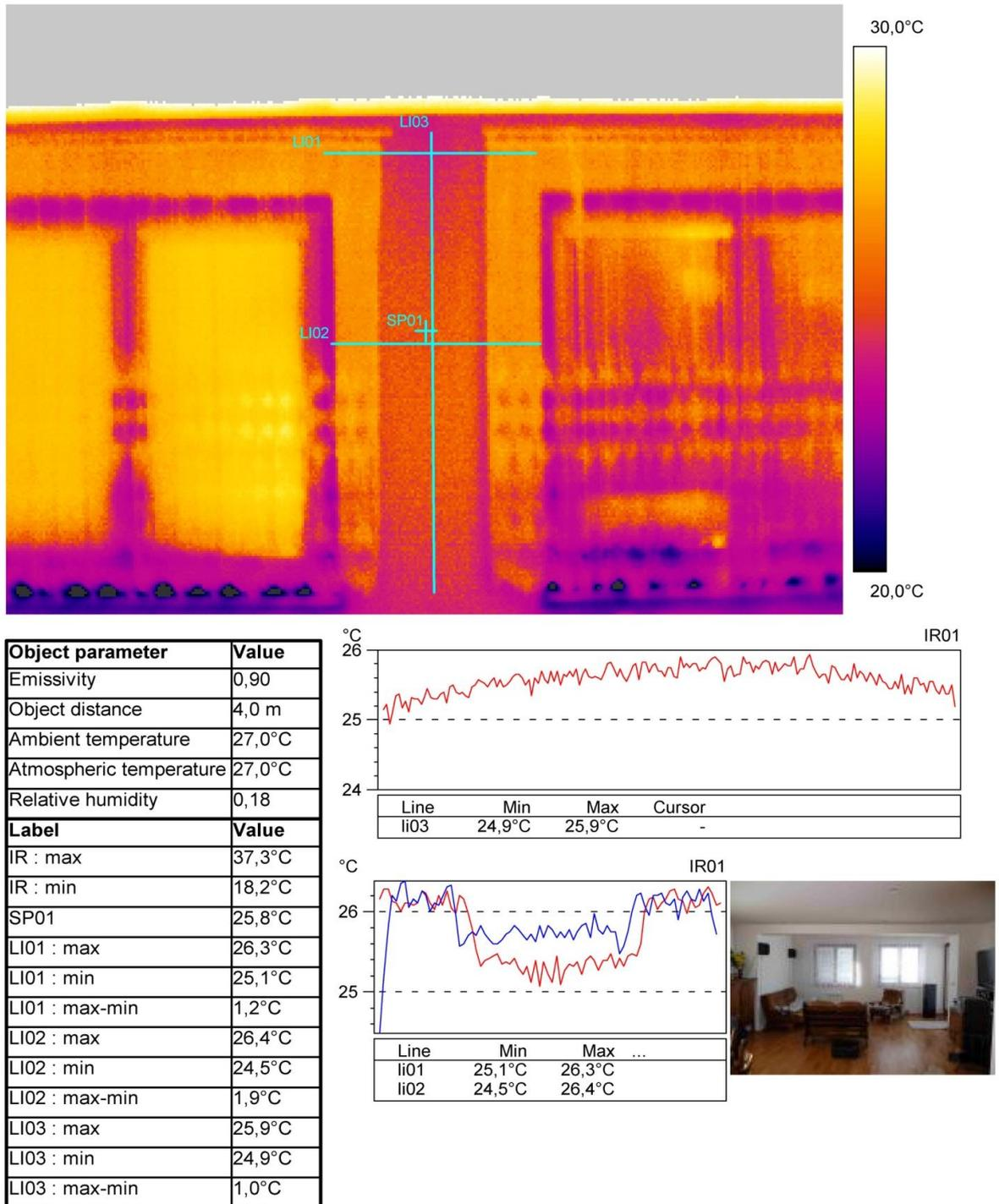
Fig. 7: Detection of the internal surface temperature differences across an internal pillar viewed from the interior. The results can be accepted (taken from [2])
