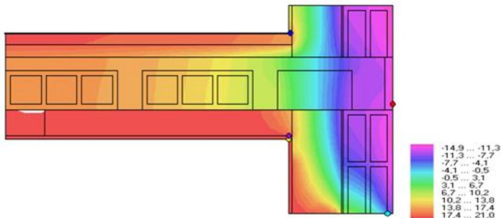
Fig. 8: Diagram of the connection between the ceiling and the outer wall
