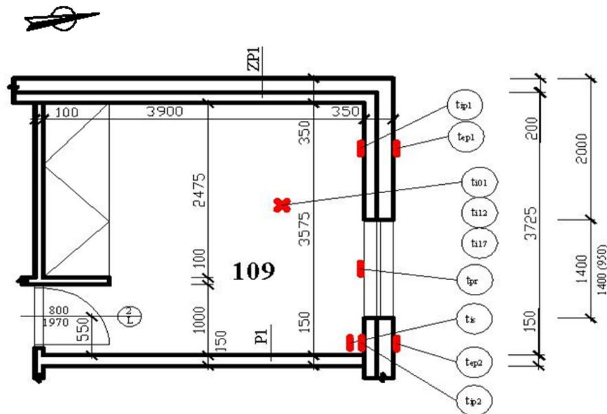
*Fig. 4: Deployment of sensors in the north-facing room on the ground floor*
