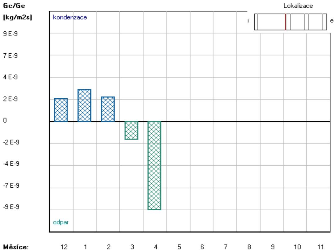
Fig. 6: Software graphical output showing a prevailing evaporation (odpar Ge) over condensation (kondenzace Gc) in months (Měsíce) of annual cycle and localization of calculations within the structure (Lokalizace)
