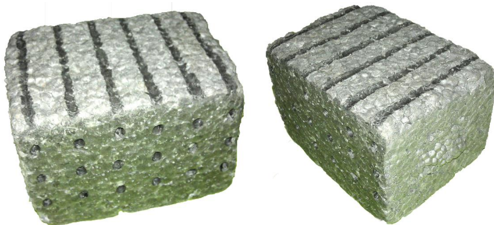
Fig. 1: Sample of perforated graphite polystyrene
