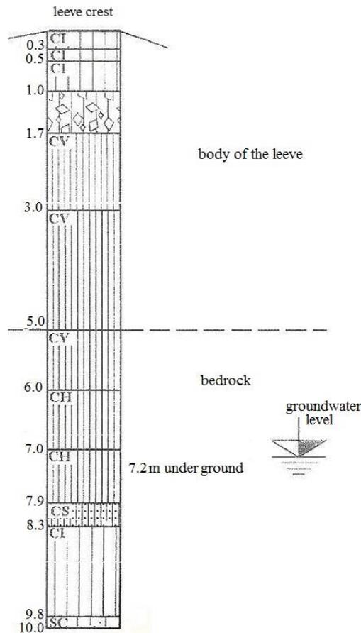
*Fig. 2: Geological profile of the levee body and its bedrock in the place of disturbance [9]*
