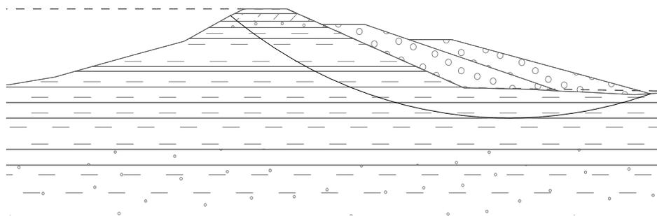
*Fig. 5: Pettersons' s method: Shear stress area after optimization - Variant III-C*
