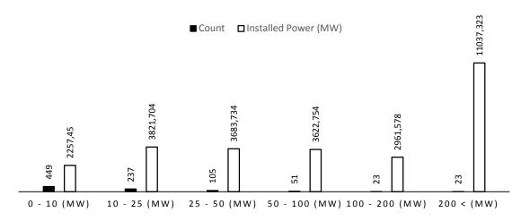
Fig. 3. Distribution of number of HPPs and total installed power by different classifications (EMRA).
