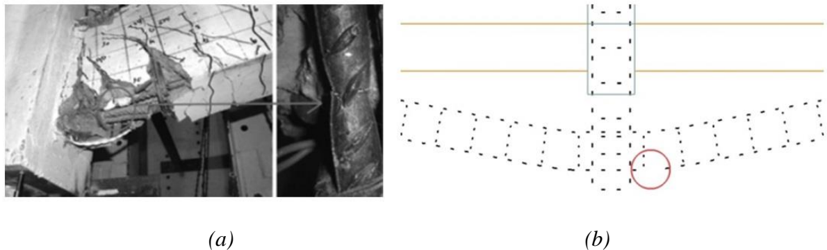
Fig. 4: Rupture of reinforcing bars in the first floor beam adjacent to the middle column: (a) experiment [17]; (b) AEM model
