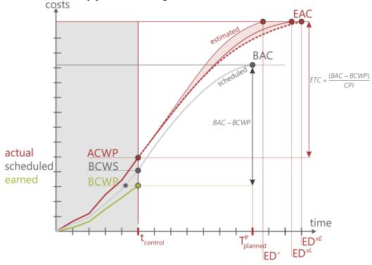
Fig. 3: Cumulative curve of actual and estimated remaining costs
