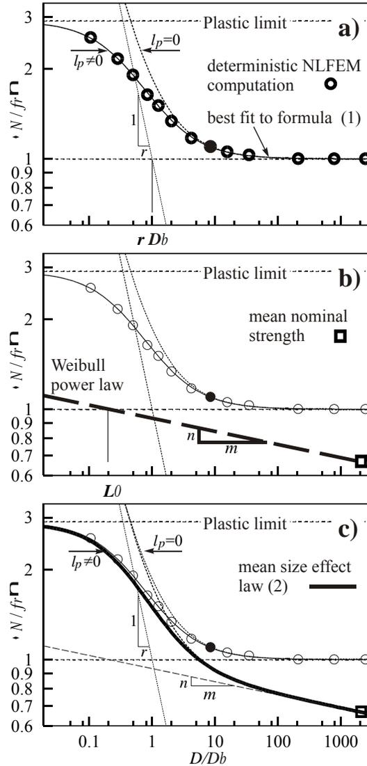
Figure 1: Illustration of the superposition steps. a) Steps 1-4 resulting in deterministic fit; b) step 5 – determination of parameter  $L_0$ ; c) final formula and nominal strength prediction for the real structural size
