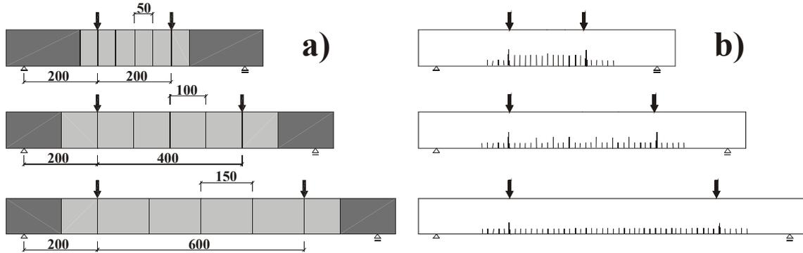
Figure 1. a) Koide's beams of bending span 200, 400 and 600 mm, series C. b) Crack patterns for deterministic calculations for the three sizes.
