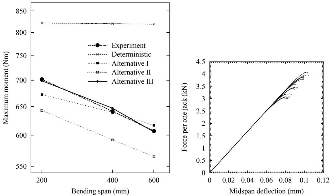
Figure 3. Left: Comparison of Koide's data and the deterministic and statistical simulations. Right: Random load-deflection curves.
