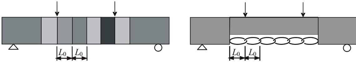
Figure 4. Simple 1-D Weibull model (chain). Left: Random variables – macroelements. Right: a statistical “chain” model driving the strength of a whole structure.
