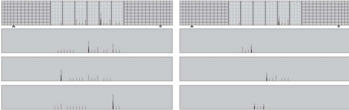
Figure 2. Macroelements (random variables) and examples of random crack initiation for the smallest beam size; left: random tensile strength only (Alternative I); right: random and highly correlated tensile strength with fracture energy.
