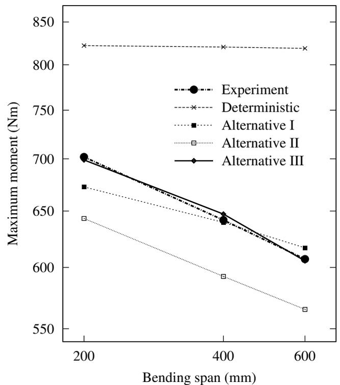
Figure 7: Comparison of means of Koide's data and ATENA deterministic and statistical simulations.
