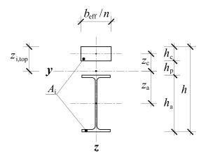
Cross section area of equivalent (ideal) all-steel section
