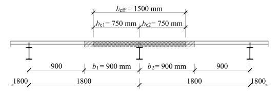
The composite section is substituted by all-steel section with reduced slab width using n ratio.
