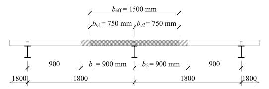
High of compressed part of concrete slab is calculated from equation where normal force in IPE section is equal to normal force in concrete slab for assumption that neutral axis passes through concrete slab.
