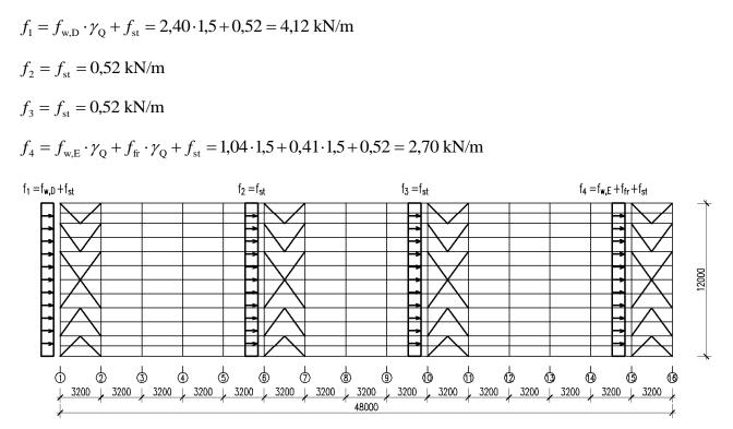
All of the transversal bracing are the same geometry and members cross sections. The most loaded of them will be analysed with load f
