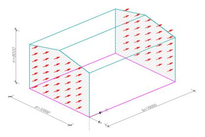
pressure coefficients for external pressure for areas D and E for geometrical ratio h/d = 8/48 = 0.166
