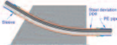
Deviation pipe protrudes from concrete at sufficient distance and is coupled to PE pipe
